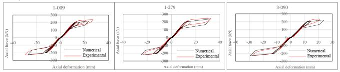
Figure 8: Experimental and numerical hysteresis response for the 3 records using the closed-loop dynamic testing
