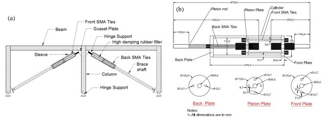
Figure 1. (a) Basic Components of a Piston Based Self-Centering brace, (b) PBSC brace components
