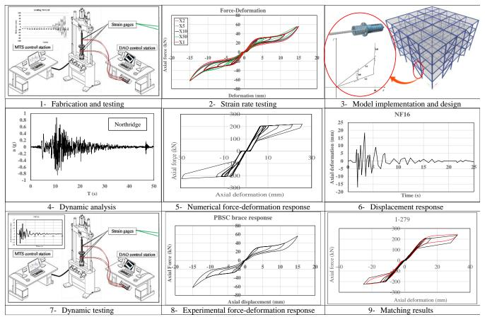
Figure 5: Closed-loop dynamic testing flow chart procedures
