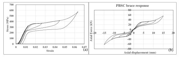
Figure 4: (a) Stress-Strain response of a single 8 mm diameter SMA bar, (b) Hysteretic response of the PBSC bracing system
