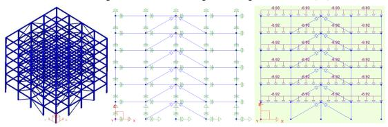
Figure 6: Three-dimensional model of the steel building, Nodal Restraint Conditions, and Uniformly distributed gravity loading on the beam for the 2D model (from left to right)
